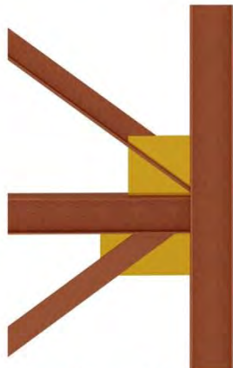
Automated Vertical Bracing Gusset Plates
