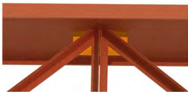
Automated Horizontal Bracing Gusset Plates
